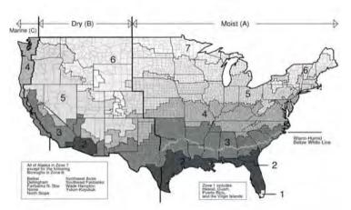
of the country, based on temperate and humidity profiles. The zones are then used to determine the required R-value of the roof, walls, slab and doors that make up the building envelope. When comparing the older and newer versions of the code, take note of the new requirement for continuous insulation within roof and wall assemblies.
