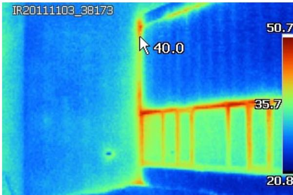
■ Thermal imaging is used to assist in the inspection for air and thermal leaks in a building enclosure.
