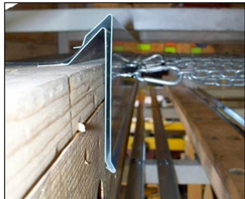
For systems having more than 4 in. of horizontal exposure, test RE-3, “Pull-Off Test for Coping,” is used. It is similar to Re-2, but it requires the wall coping system to be loaded in both an upward direction (on the horizontal face) as well as an outward direction (on one of the
