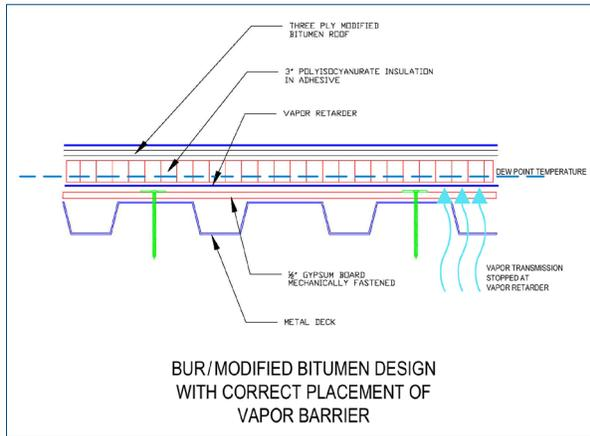
Two of the most popular products used as vapor retarders in the roofing industry are polyethylene plastic sheets and two-ply fiberglass felts adhered in hot asphalt. But any material that has a permeability rating of 1.0 or less, in accordance with ASTM E 1745, is acceptable as a vapor retarder.
