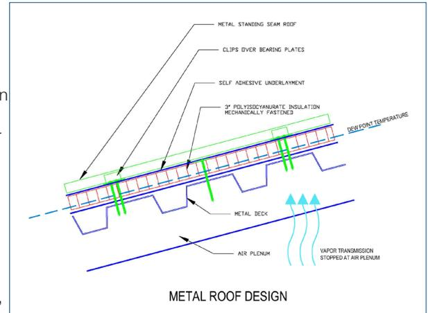
below, an air plenum can be used to ventilate the space between the interior finish and the roof deck where the screws are penetrating. In this way, the chance of vapor drive up the fasteners is eliminated. In higher sloped metal roofs, this air plenum would be the unheated attic space above the ceiling and insulation. In lower sloped metal roof constructions, an air plenum may be created with a drop ceiling.
